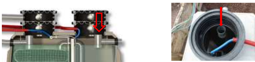
Fig 6b : Sampling Tee fitting inside an Oxyfix® 7,8-9,10-12,13-14,15-17,18-20 ou 21-27PE unit
