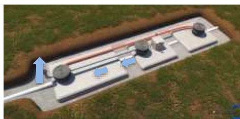
Fig-25: Vent pipe fitted to a three-tank Oxyfix® C-90 unit
